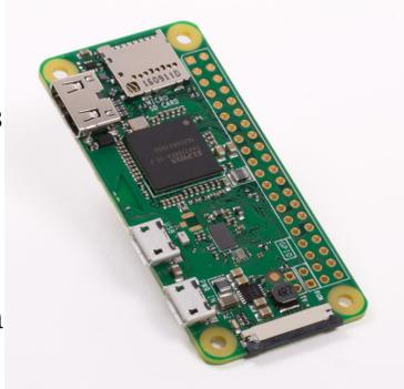
The low-profile (2.6" x 1.2" x 0.2") Pi Zero technically has a full-size GPIO header, but the pins have to be soldered on by the user if they are needed.
